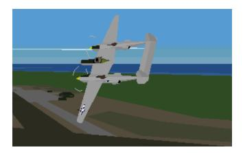
Nicknamed the "Fork-Tailed Devil" by its foes, the Lockheed P-38 Lightning was highly regarded by the pilots that made it famous. One of the few American fighters to mount a cannon, the Lightning had an additional gunnery advantage... all of its weapons mounted in the nose, largely eliminating convergence issues.
