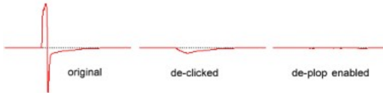
Fig.4: Large click followed by resonance tail (left), de-clicked without (middle) and with (right) the De-Plop Filter .
