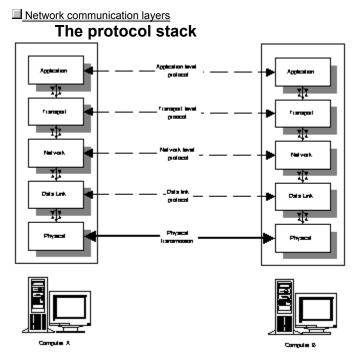
The figure shows the layers of a protocol stack, based on a simplification of the OSI Reference Model of network communications.
