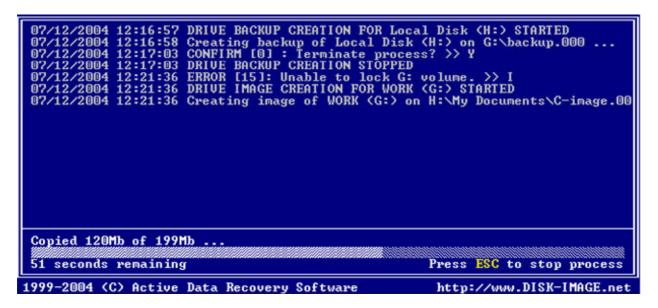
Created *C-image.DIM* file is a text file containing image parameters. Since files on FAT volumes are limited to 2GB, image file will be automatically splitted into 2GB data chunks. Image Data chunks would be: *C-image.000, C-image.001, C-image.002,* etc...
