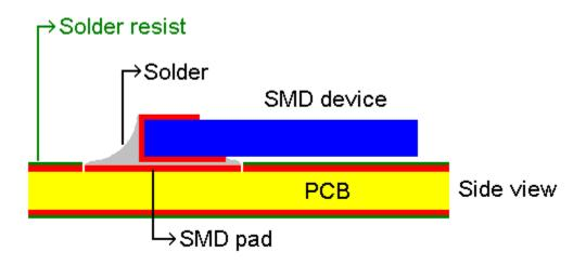
In the above figure a SMD pad is shown after soldering. By applying heat on top of the PCB, SMD devices will be soldered using the solder paste on the pad as the solder.
