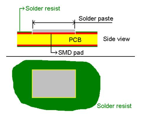
In the above figure a SMD pad with solder paste is shown.
