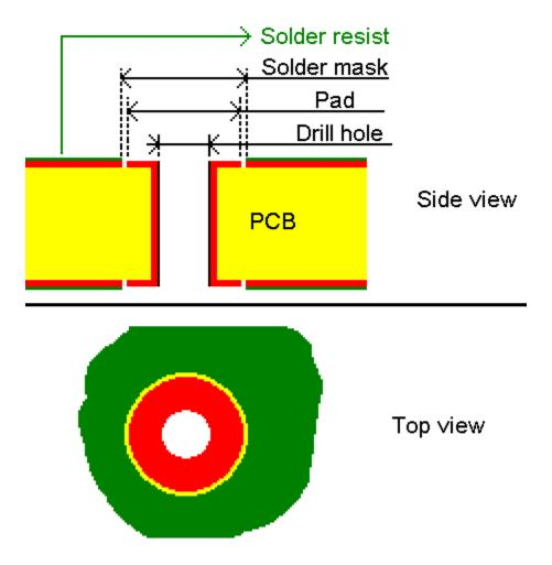
In the above figure a through hole pin is shown.
