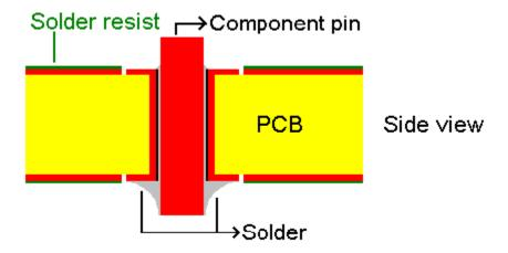
After the bottom side of the PCB has gone through a solder bath, all copper areas at the bottom of the PCB are soldered. The copper areas on the bottom PCB side which are covered with solder resist, are not soldered.
