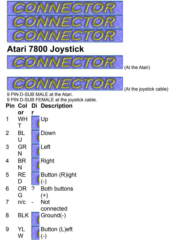
Note: Direction is Computer relative Joystick. Note: Connect Direction and Button(L/R) to Ground for action. And Both Button to Button L and Button R for action.
