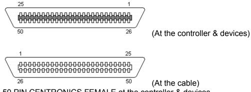
50 PIN CENTRONICS FEMALE at the controller & devices. 50 PIN CENTRONICS MALE at the cable.
