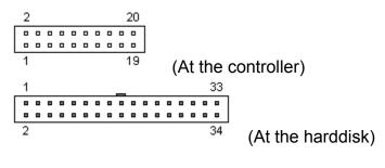
34 PIN IDC MALE at the Controller.20 PIN IDC MALE at the Controller.34 PIN IDC FEMALE at the Harddisk.20 PIN IDC FEMALE at the Harddisk.
