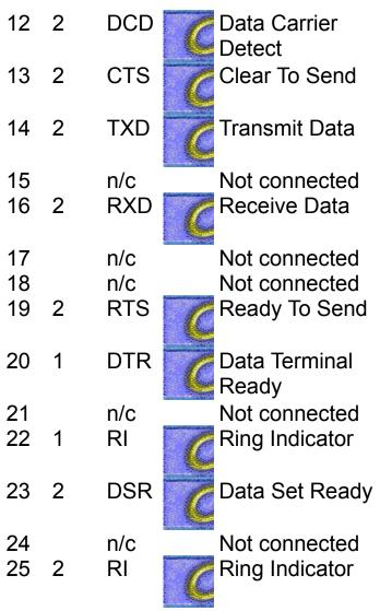
Note: Direction is DTE (Computer) relative DCE (Modem).
