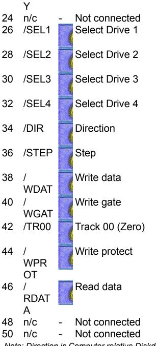
Note: Direction is Computer relative Diskdrive. Note: All odd pins are GND, Ground.
