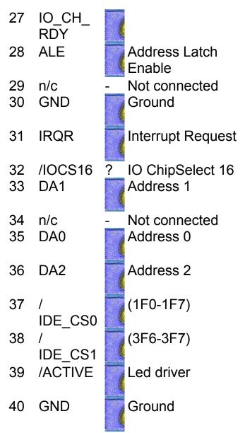
Note: Direction is Controller relative Devices (Harddisks).
