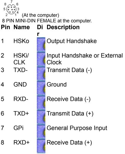
Note: Direction is DTE (Computer) relative DCE (Modem).
