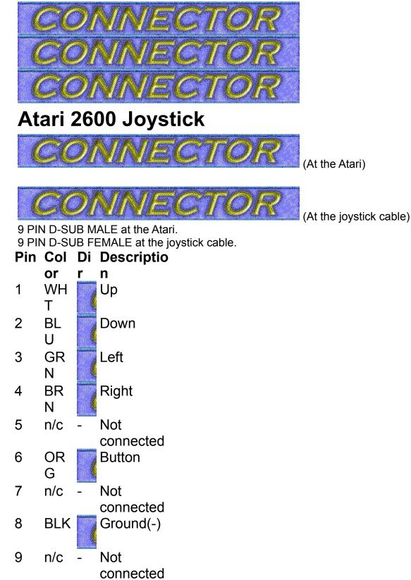
*Note: Direction is Computer relative Joystick. Note: Connect Direction/Button to Ground for action.*
