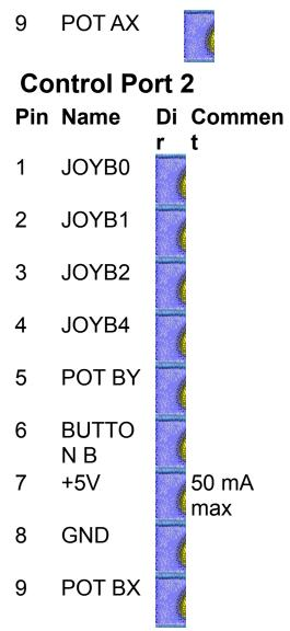
Note: Direction is Computer relative Device. Note: Pot is a linear 470 kOhm (±10 %)
