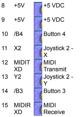
Note: Direction is Computer relative Joystick. Note: Use 100 kohm resistor.
