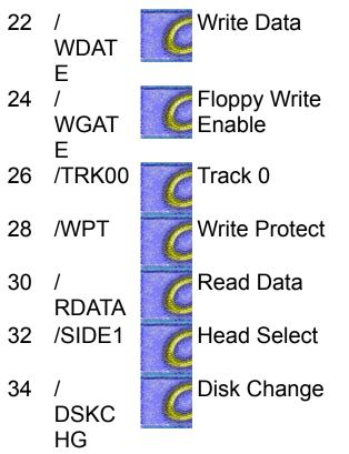
Note: Direction is Computer relative Diskdrive. Note: All odd pins are GND, Ground.
