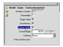
Notice how the object's appearance improves. When Crease control was off, AXEL was trying to smooth out all the object's corners, even corners that were not meant to be smooth, like the top edges of the holes. When Crease control is on, AXEL does not try to smooth out 90-degree angles.
