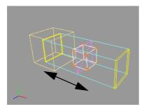
6. To make the cube slide toward the front along the Z axis, make sure the small cube is at position (0,0,0), then rotate the blue slider joint in the Top viewport.
