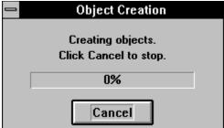
After you create a gauge, you set its value using the **PercentGaugeValue** property. Set it equal to a number from 0 to 100 to have the gauge show the appropriate position. For example, if the operation is 53% complete, the following statement makes the gauge show that value.
