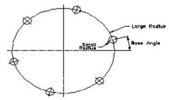
The Create Circular Pattern utility creates a pattern of small circles at a given distance from a given point.
