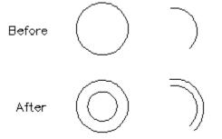
The Create Concentric Arcs and Circles command will create duplicate copies of arcs or circles as a specified distance from the radius. All attributes of the original arc/circle are recreated. In the case of arcs the starting and ending angles of the new arc will be the same as the original arc.
