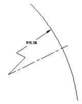
The Foreshortened Dimension utility creates a foreshortened radial dimension. A foreshortened dimension is used to indicate the radius of an arc when the center of the arc is either off the drawing or so far removed from the arc that using a standard radial dimension is impractical.
