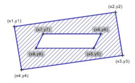
If a surface is drawn with a non-solid line pattern, this line pattern has to be continued during each curve. A surface may contain up to 1000 nested curves made of up to 2000 data blocks in total.
