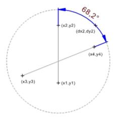
The image above shows an angle dimension created using the settings described above. The points (x1,y1), (x2,y2), (x3,y3) and (x4,y4) define the two edges of the angle. The dimension line has a distance of 10 mm to the point (x4,y4).
