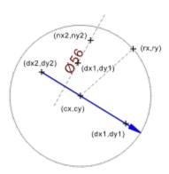
The image above shows another diameter dimension. It was created using settings similar to the settings described above, but *LineType* was set to 0x0002, so the dimension line has only partial length and a single arrow.
