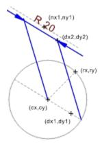
The image above shows a radius dimension created using the settings described above. The points (cx,cy) and (rx,ry) define the radius to be dimensioned. The dimension's orientation is determined by the first dimension line definition point (dx1,dy1).
