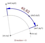
The image above shows an arc length dimension created using the settings described above. The points (cx,cy), (rx,ry), (ax1,ay1) and (ax2,ay2) define the circluar arc to be measured. The dimension line has a distance of 10 mm, the point (dx2,dy2) determines its position.
