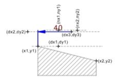
The image above shows another distance dimension. It was created using settings similar to the settings described above but LineType was set to 0x0002, so the dimension line has only partial length and a single arrow.
