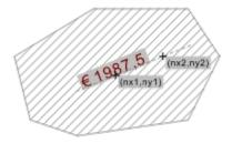
The image above shows an area dimension created using the settings described above. The points (nx1,ny1) and (nx2,ny2) place and rotate the dimension number.
