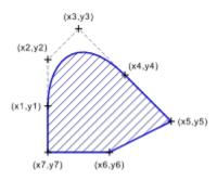
If a surface consists of multiple curves they will be filled alternately, i.e. only areas overlapped by an *odd* number of curve's insides will be filled. If, e.g., a small round curve lies inside a large one, this small round curve will be transparent, as its inside in overlapped by two curves (*even* number!):
