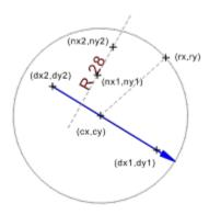
The image above shows another radius dimension. It was created using settings similar to the settings described above but *LineType* was set to 0x0002, so the dimension line has only partial length and a single arrow.
