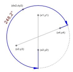
The image above shows another similar angle dimension but now dimension line definition point (dx2,dy2) was placed somewhere else, so now the upper left angle is measured.
