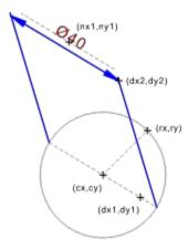
The image above shows a diameter dimension created using the settings described above. The points (cx,cy) and (rx,ry) define the diameter to be dimensioned. The dimension's orientation is determined by the first dimension line definition point (dx1,dy1).
