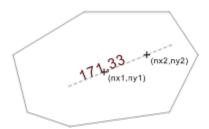
The image above shows a perimeter dimension created using the settings described above. The points (nx1,ny1) and (nx2,ny2) place and rotate the dimension number.
