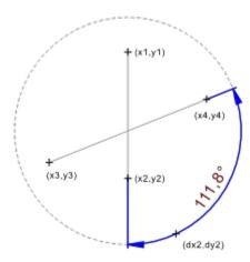
The image above shows a similar angle dimension, but the end-points of the first edge are placed vice versa. As (x2,y2) now lies below (x1,y1), the dimension starts below the virtual intersection point. According to the dimension line definition point (dx2,dy2), the lower right angle is to be measured.
