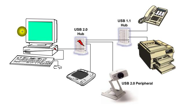
Figure 2. Future USB 2.0 System Configuration
