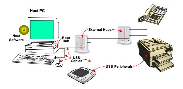
Figure 1. USB 1.1 System Configuration
