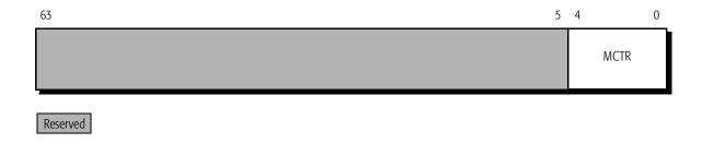
Figure 31. Machine-Check Type Register (MCTR)
