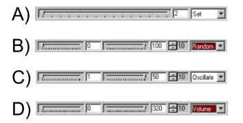
**Set** - The value for the control is set to whatever value is indicated by the slider component. The controls in "A" (above) demonstrate a "Set" source. In this case, the value will be set to 2.
