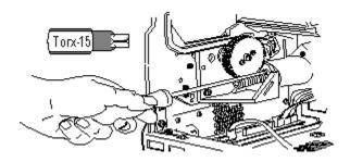
3- Pull the media motor out trough the back of the plotter.
