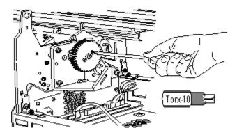
5- Remove the drive-roller gear from the drive-roller shaft.
