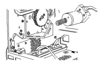
4- Remove the two screws that secure the drive-roller gear to the drive-roller shaft.
