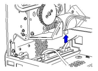
2- Remove the two screws that secure the media motor to the media-motor mount.
