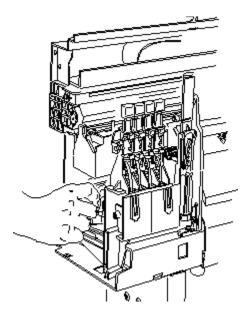
2- Remove the screw that attaches the service station to the left side plate.
