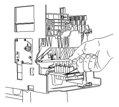
3- Slide the service station to the left, and remove it from the plotter.
