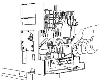
3- Slide the primer to the left, and remove it from the plotter.
