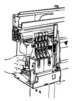
2- Remove the screw that attaches the primer to the left side-plate.
