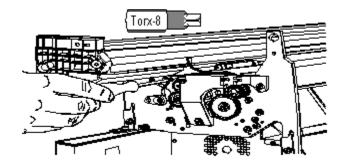
7- Remove the screw from the plastic bail gear.
