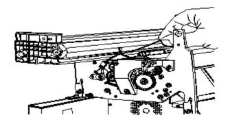
3- Release the cable from the bail-gear assembly.
