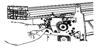
6- Loosen the screw from the top of the bail-gear assembly.
