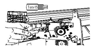
8- Pull the bail gear assembly out from the plotter.
