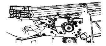
5- Remove the spring from the bail-gear assembly.
