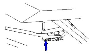
8- Refasten the media-sensor cable in its clip, making sure that it does not obstruct motion of the media-sensor flags.
