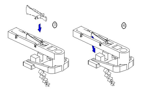
5- Insert the long arm of the media-sensor assembly into the slot at the back of the entry platern as shown.
