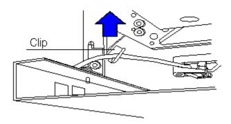
3- Remove the media-sensor assembly from the plotter.
