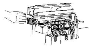
6- Loosely fit, but do not tighten , the washer and screw to retain the encoder strip.
