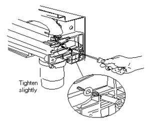
9- Slightly tighten the scew on the left side.
