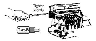
10- Slide the carriage back and forth the length of its travel to ensure free movement. The encoder strip should not bind or rub on the carriage.
