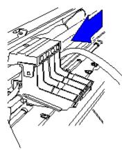
4- Temporarily, rest the loose strip safely on the drive roller.
