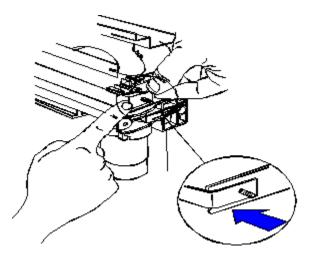
CAUTION In the following two steps, avoid distorting the encoder strip while you tighten it.
