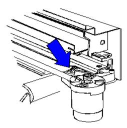
b) The other is a flat metal spring attached underneath the motor. Position it *underneath* the chassis beam.
