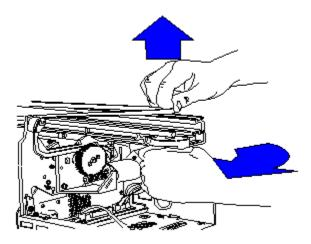
3- Slightly rotate the motor on its hinge until the indicated part of the black plastic is parallel with the side of the chassis beam.
