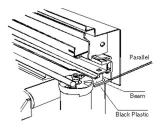
4- Pull the motor out to the right of the plotter. **Note:** The motor may be stiff.
