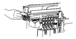
8-Carefully pull the encoder strip to the right, through and out of the carriage assembly.
