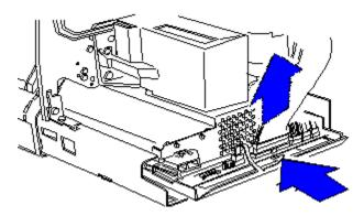
2- Disconnect the trailing cable from the guides on the right bracket.
