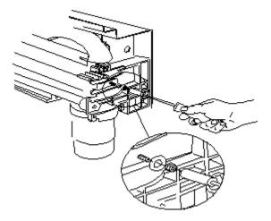
5- Remove the screw and washer that secure the encoder strip to the left bracket.
