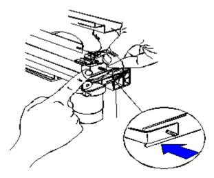
7- Carefully release the encoder strip from the left bracket.
