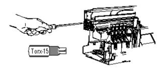
6- Compressing the encoder-strip spring to release the tension on the encoder strip, carefully release the encoder strip from the pin on the spring.
