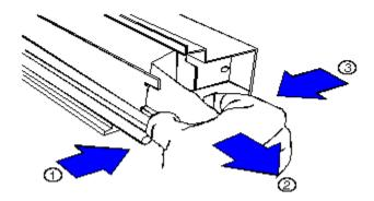
3- Fold the trailing cable upwards and store it on the trailing-cable guide.
