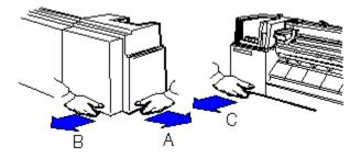
2- Pull the end-cover up, and remove it from the plotter.
