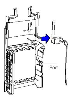
4- Detach the sensor cable from the COVER connector on the main PCA, and unclip it from the side of the electronics module.
