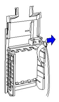
3- Raise the plastic clip and remove the sensor.
