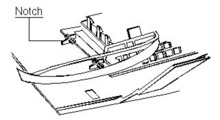
Push the front panel from the outside, to check whether it is correctly installed.
