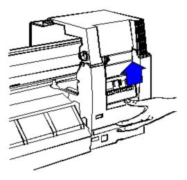
5- Inside the end-cover, press the two indicated tabs towards each other, and remove the front-panel assembly from the end-cover.
