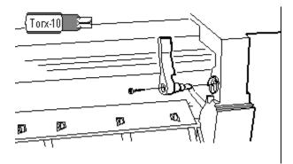
2- Pull the plotter on/off switch out of the end-cover.
