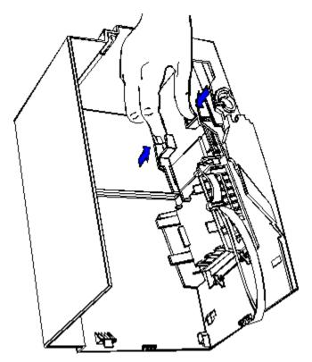
6- To be able to easily use the front panel, when the right end-cover has been removed, slide the front-panel assembly onto the metal base of the plotter as shown.
