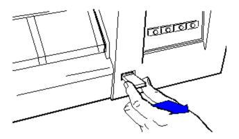
3- Release the three clips at the bottom of the end-cover: first the side clip, them the front and back clips.
