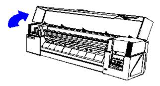
2- Push the right-hand side of the cover slightly back, so that the rightmost hinge uncouples.
