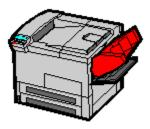
The envelope feeder is an additional input source designed specifically for feeding multiple envelopes. You must add this accessory in the driver by selecting it from the Accessories screen if you are not in a <u>bi-directional communications</u> environment.
