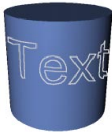
Here text is projected, perpendicularly to the XY plane, onto a cylinder
