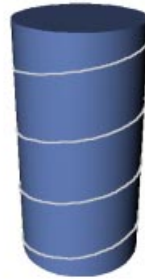
Here is a helix projected in the X and Z directions on to a cylinder
