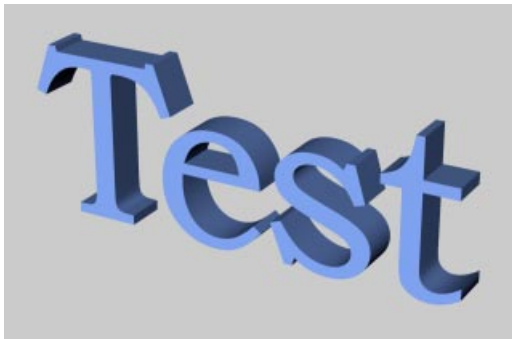
A spline converted to a 3D object with holes automatically created
