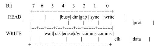
Bits DTR and CTS are used by the RS232 interface. The WAIT bit is used by the Network to synchronise, GAP, SYNC, WR\_PROT, ERASE, R/\_W, COMMS CLK and COMMS DATA are used by the microdrive system. If the microdrive is not being used, the COMMS DATA output selects the function of bit 0 of out-port F7:
