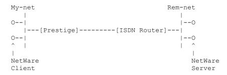
The Prestige can place calls to a remote ISDN router to Bridge IPX packets. In this configuration, the stations on the LAN (My-net) will have access to the IPX NetWare server and other network resources available on 'Rem-net'. Note that in this setup, there is no NetWare server on 'My-net'.
