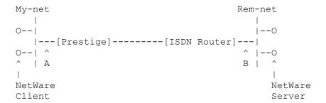
The Prestige can place calls to a remote ISDN router to negotiate IPX routing. In this configuration, the stations on the LAN (My-net) will have access to the IPX NetWare server and other network resources available on 'Rem-net' and vice versa. Note that in this setup, there is no NetWare server on 'My-net'.
