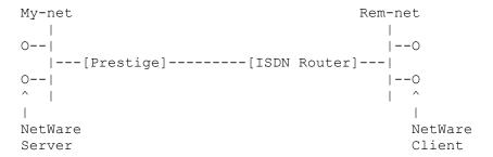
The Prestige can accept calls from a remote router to Bridge IPX packets. In this configuration, the stations on the remote network (Rem-net) will have access to the IPX network resources available on 'My-net'.
