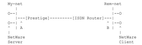
The Prestige can accept calls from a remote router to negotiate IPX routing. In this configuration, the stations on the remote network (Rem-net) will have access to the IPX network resources available on 'My-net' and vice versa.
