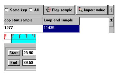
Clicking **Import value** while the **Start sample** or **Loop start sample** fields are selected in the data display grid causes the value in the **Start** edit box of the WAView window to be copied into the grid (after a unit conversion, if needed).
