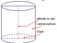
The bases are circles and the line between the centers of the bases is the cylinder's **axis**. Since the axis is perpendicular to the to the bases it is coincident with the **altitude**. See also Mensuration.
