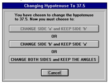
When the hypotenuse is changed, the geometry of the triangle must also change. The dialog is necessary because WAM+ needs to know whether you want to change side 'a', change side 'b', or change both sides and keep the existing angles.
