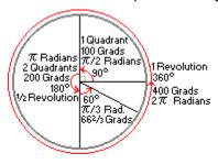
The diagram above shows a circle divided into sections forming a 60° <u>acute angle</u>, a 90° <u>right angle</u>, and a 180° <u>straight angle</u>. The circle itself, of course, is 360° or 1 revolution. A fourth type of angle, the <u>obtuse angle</u>, is not shown.
