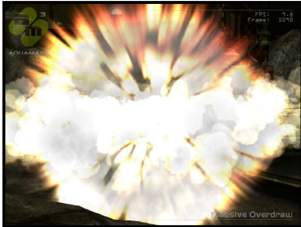
Picture 9: Massive overdraw caused by alpha blended particles
