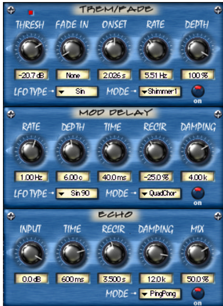
Figure 40. The TremModEcho plugin contains three modules.
