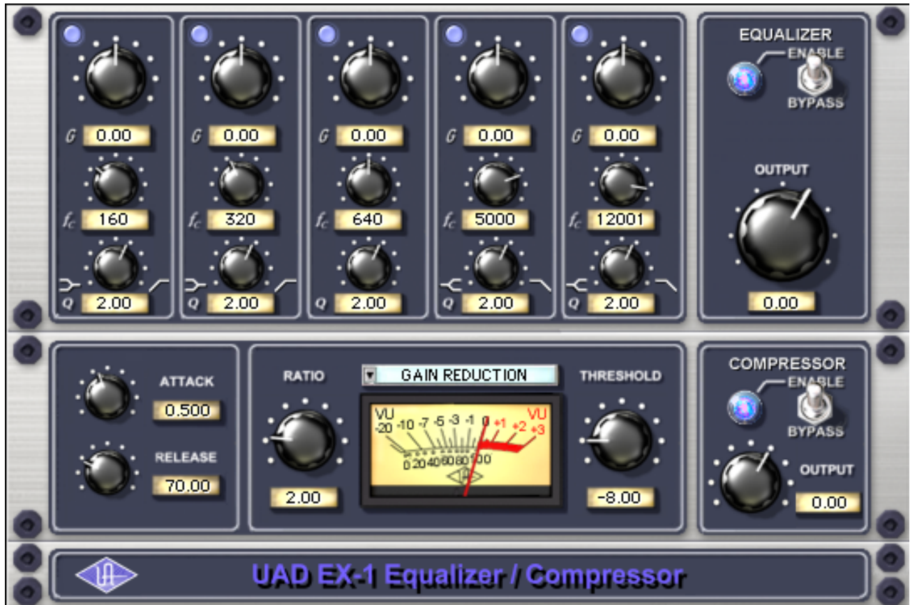
Figure 29. The EX-1 EQ/Compressor plugin window.
