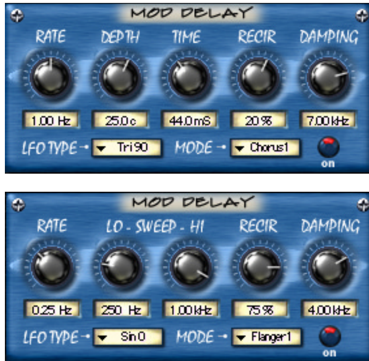
Figure 42. The Mod Delay module. The label and function of the second two knobs depend upon the Mode menu selection.
