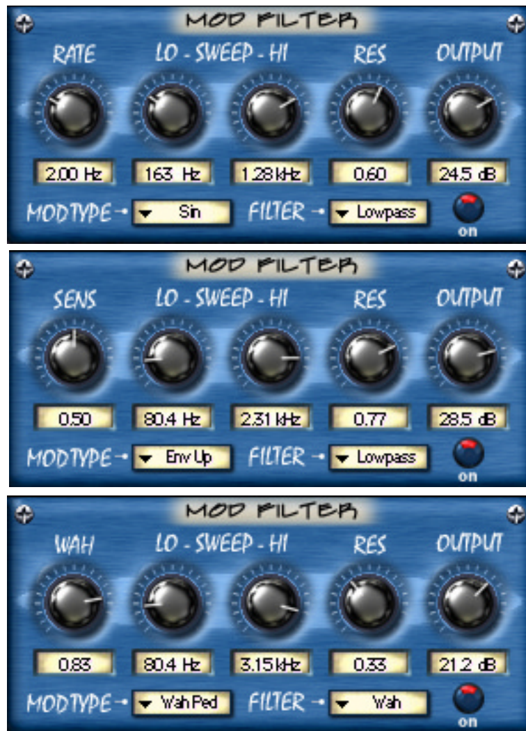
Figure 39. The Mod Filter plugin window. The label and function of the first knob depends upon the Mod Type menu selection.
