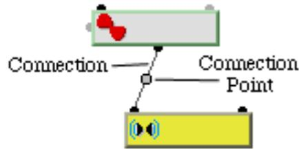
A signal will flow from the output of the upper operator into the first input of the lower operator. Each connection has a connection point. You can control the volume of the connection using the connection point by hooking an operator that makes a volume output to the point.
