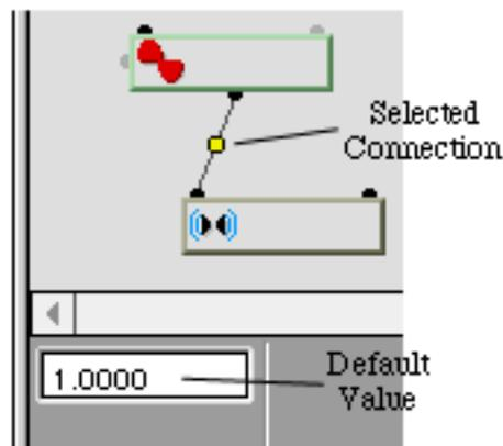
If you were to change the default value here to 2, the output of the Wave operator would be multiplied by 2 before it was delivered to the next operator.
