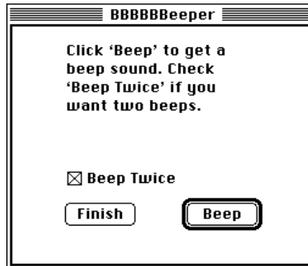
The smarter dialog as it appears when used by Open Prolog. The check box has been clicked.
