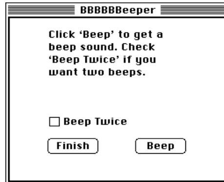
This is a movable modal dialog containing four items - two buttons, a piece of static text and a check box.
