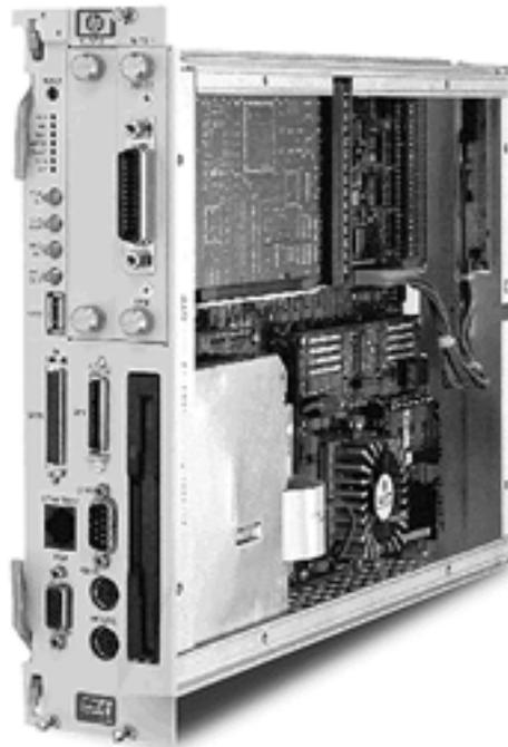
Figure 1-1. The HP E623x VXI Pentium Controller
