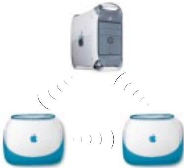
Instead of communicating through a wired network, all AirPort-equipped Macintosh computers can communicate directly with each other without cables or complicated networking hardware. It's a much simpler way to transfer files to other computers without using floppy drives, cables, or infrared equipment. You can share files and play games wherever you happen to be.
