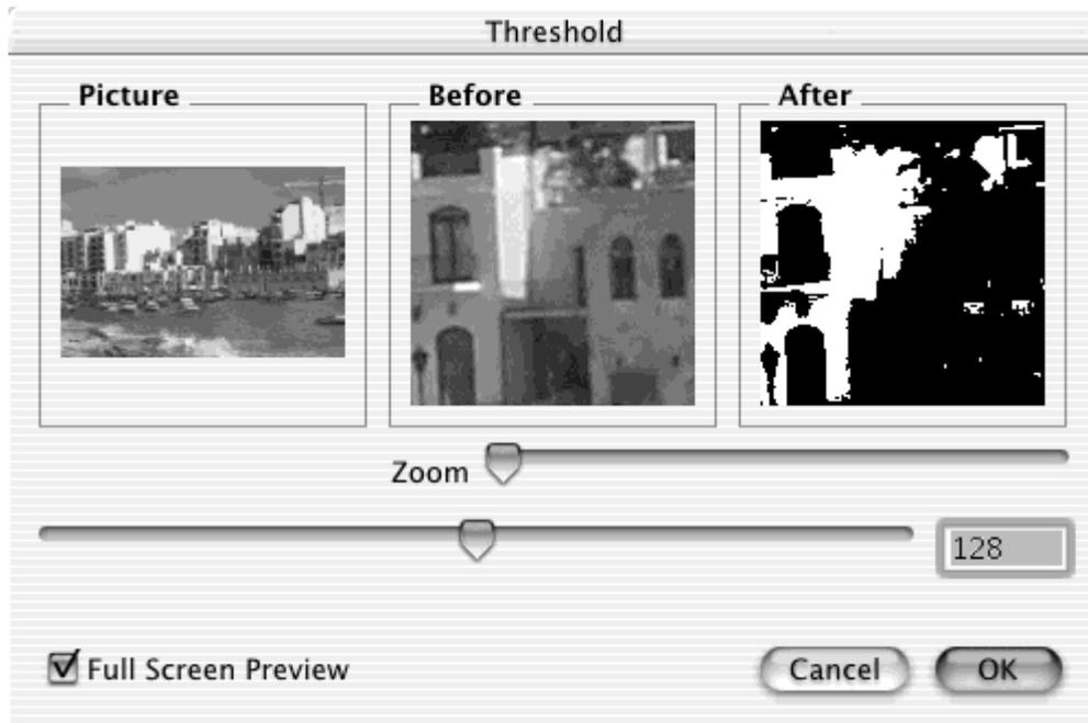
Converts the picture directly to a black & white picture. Every pixel value in the original that has a level lower than the threshold value will be made black in the destination picture.
