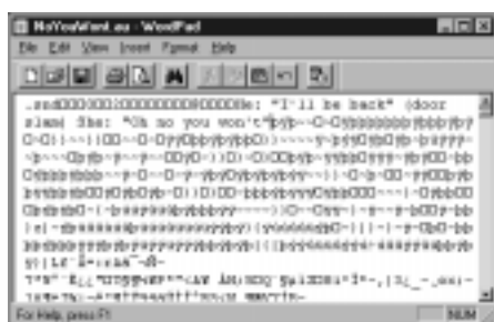
Figure 2-7 The .snd at the beginning of the file tells you this is an AU file (or a NeXT SND file).
