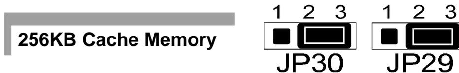
On mainboard integrate 256KB pipeline burst cache mounted, or a primary 256KB pipeline burst cache module in the CELP socket.
