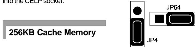
On mainboard integrate 256KB pipeline burst cache mounted, or a first 256KB pipeline burst cache module in the CELP socket.
