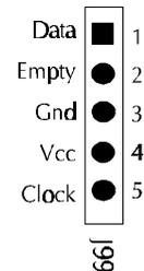
HOT-555A mainboard supplies two types of optional PS/2 mouse adapter cable, type 1 with 6-holes plug which hole 2 and hole 6 are wireless; type 2 with 5-holes plug which hole 2 is wireless.
