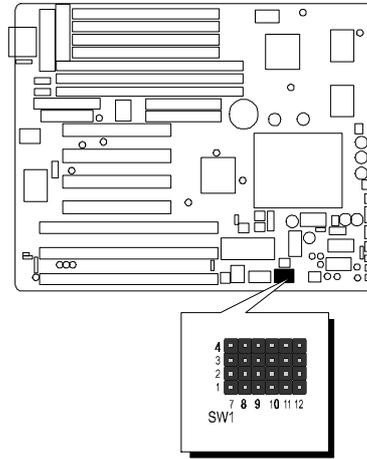
**Voltage Auto-Setting** -- Inserting jumper pack on jumper group row 2/3 of SW1. Setting to **AUTO** on "**CPU Voltage**" item in Chipset Setup Feature of BIOS Software. System will auto-detect CPU type and assign proper voltages.
