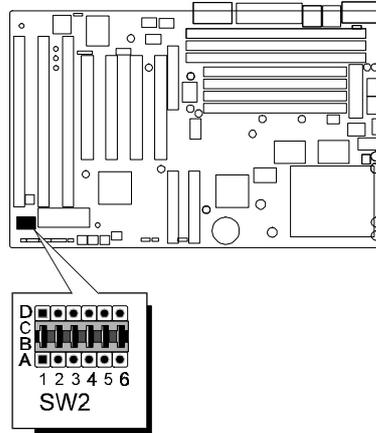
**Voltage Auto-setting** -- Inserting jumper pack on jumper group row B/C of SW2. Setting to **AUTO** on "**CPU Voltage**" item in Chipset Setup Feature of BIOS Software. System will auto-detect CPU type and assign proper voltages.
