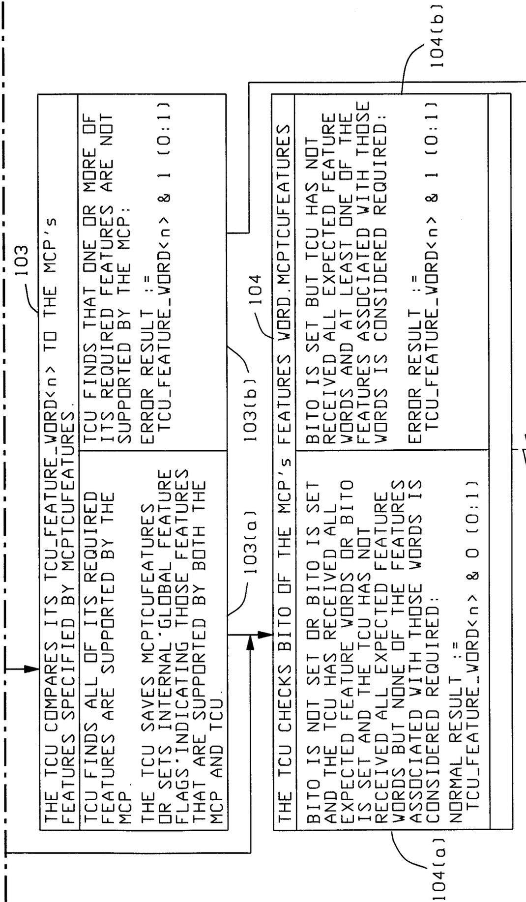
FIG. 3(a) RETURN TCU\_FEATURE\_WORD<n> RESULT TO MCP
