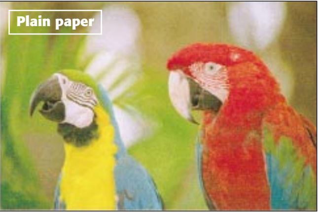
The Lexmark 7000's plain paper performance is a little more even than the Stylus Color 400's, with colours being a touch brighter. There's also less soak-through of ink on the page, though neither printer causes any paper rippling.
