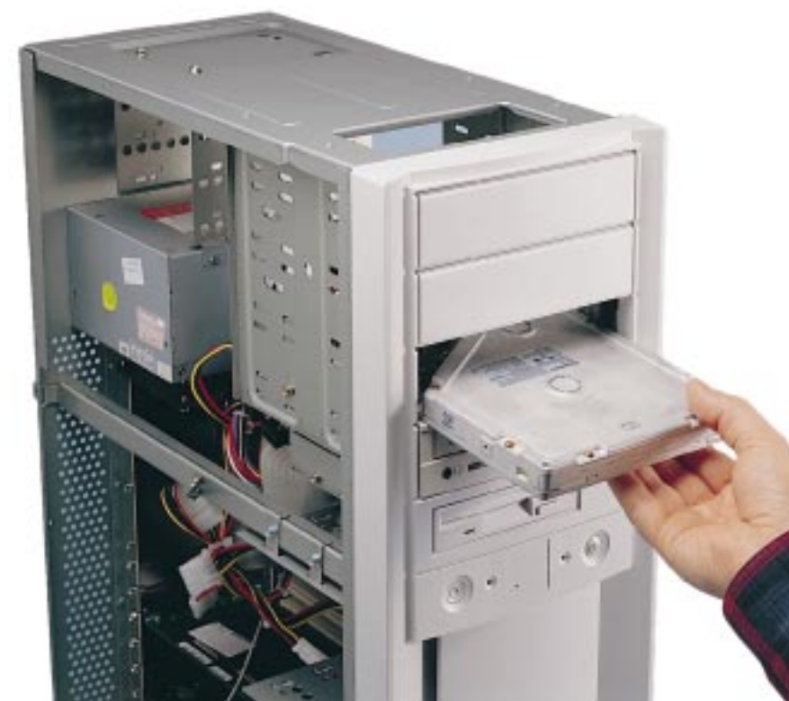
The Quantum Bigfoot, like most IDE hard disks, requires a 5.25in drive bay
