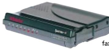
computer equipped with a modem. Virtually all modems allow you to send and receive faxes, and many of the more recent ones can act as telephone answering machines by recording messages onto the PC's internal hard disk.
