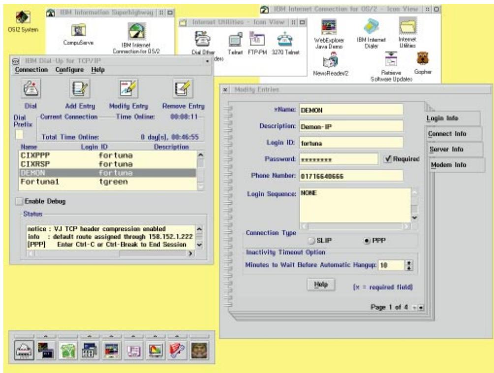
Setting up IBM's catchily-named Dial Other Internet Provider utility. It's important to get every detail correct in order to avoid connection errors
