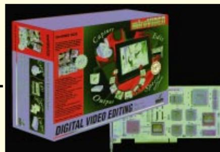
gives 24-bit colour (as with other cards) when grabbing moving video, but it's also capable of 32-bit colour still-image capture — as are some of the latest flatbed image scanners. It accepts S-Video as well as composite signals (all three TV signal standards: PAL, NTSC and SECAM are supported).
