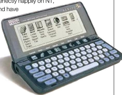
Use an extra serial port to connect your Psion and make use of its PsiWin software
