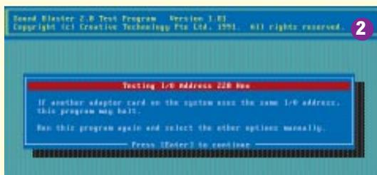
**Fig2** The SoundBlaster comes with a simple diagnostics program, TEST-SBC.EXE, which checks for hardware conflicts and plays some sample sounds to make sure that all is well
