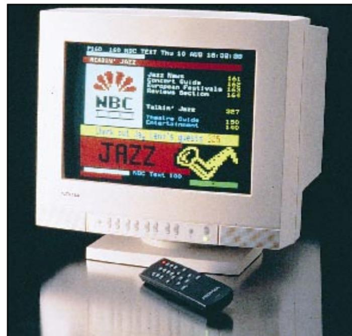
The Nokia Valuegraph 417TV is a 17in computer monitor which doubles as a remote-controlled colour television with fast-text Teletext.
