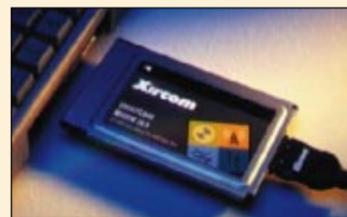
The Xircom Creditcard Modem 28.8 is a V.34 PCMCIA card modem offering uncompressed data rates of up to 28,800bps, as well as a 14,400bps fax capability.
