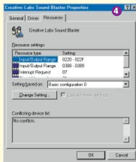
auto-identify your new sound card. When it does, you'll be prompted for the Windows 95 installation disks or the manufacturer's driver disks. You can then check its correct installation by clicking on the "System" in Control Panel, then on the "Device Manager" tab and selecting the "Sound, video and game controllers" entry on the device tree.
