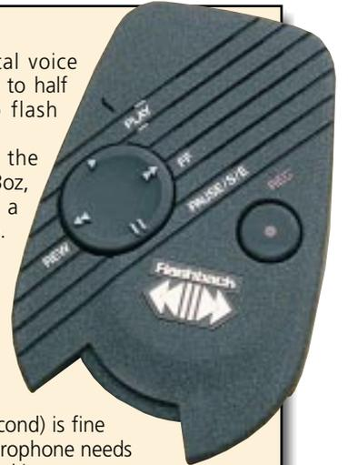
Recordings can be edited on the Flashback itself but it comes with a device for downloading audio to a notebook PC. The 'Voicelink' is a PC Card device that takes the Flashback's flash memory card and provides it as a virtual disk drive. Software is supplied to read and write recordings from the memory card and the Voicelink can also double as a sound card using its built-in speaker.
