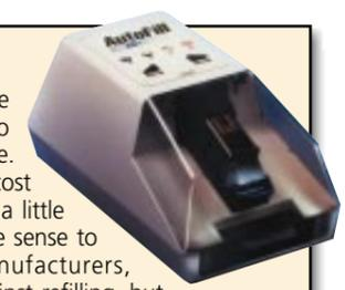
Unlike other systems that require you to inject ink into the cartridge using a syringe, the mains-powered Autofill 500 completely automates the process. Empty cartridges are locked in position, the lid closed and then refilled with the press of a button. There's no mess, and the device only dispenses as much ink as is needed. Ink is stored in a replaceable cassette, which is good for three refills.
